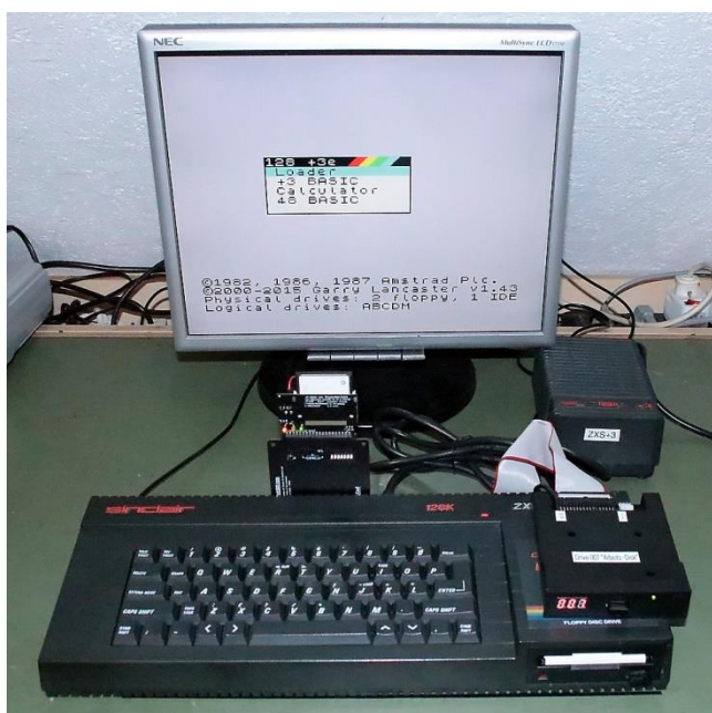
Spectrum+3 attached with 8BitIDE and Gotek drive
